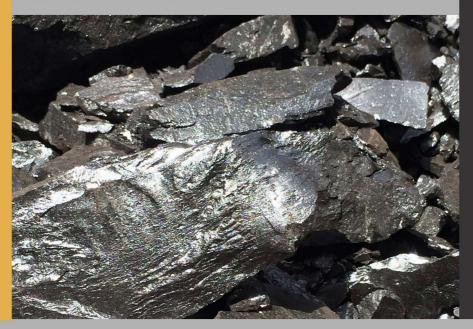
The presence of nitrogenous compounds in Gilsonite makes it highly adhesive and increases its resistance to oxidation as well. Studies show that adding 5 to 15% gilsonite to tar significantly increases its hardness and deformation resistance, along with a significant effect on its viscosity and elasticity.
